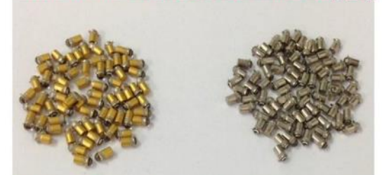
Before Gold stripping After Gold stripping
