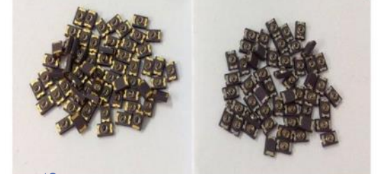
Before Gold stripping After Gold stripping
