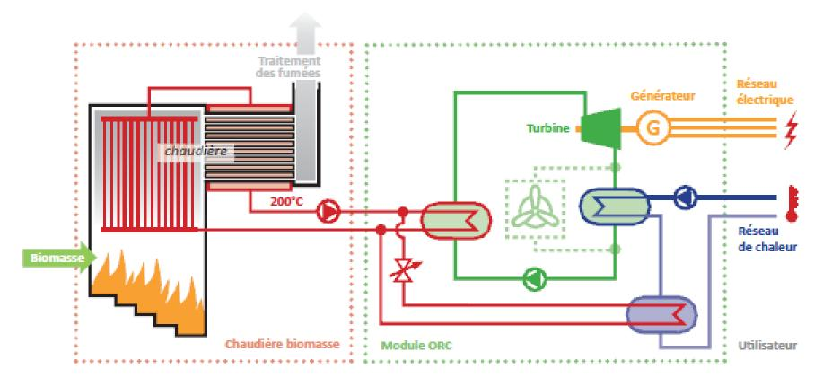
500KWe — 5MWth – for heat or for cold with and absorption system.
