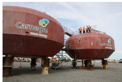
CETO 5, 3 x 240kW array Power & water production Western Australia.
