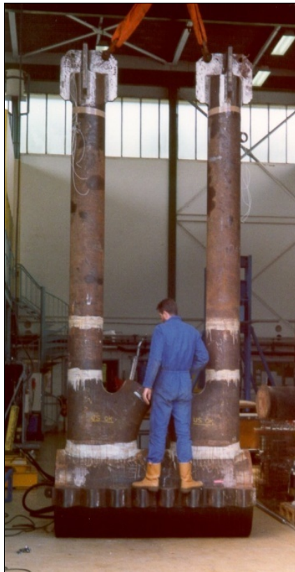
Fatigue test on a piece of an offshore structure
