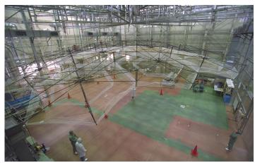
Onboard large deployable antenna reflector of ETS-VIII
