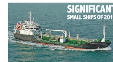
GAZPROMNEFT NORTHWEST: Turkish-designed and built, oil- and chemical-carrying bunkering tanker
