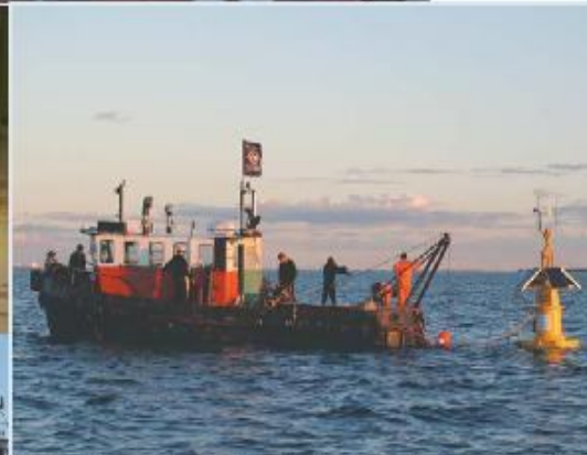
Monitoring buoys will relay the dissolved oxygen levels, temperature and conductivity levels in Cockburn Sound in real time. Data is sent to the plant site via GSM Mobile and radio.
