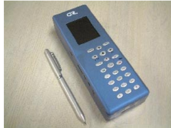
Developed handheld phone for ETS-VIII experiments
