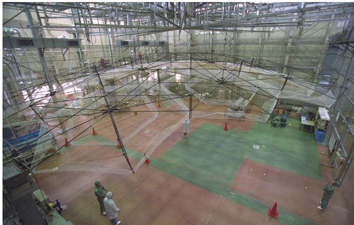
Onboard large deployable antenna reflector of ETS-VIII
